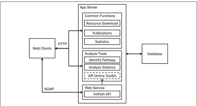
**Figure 4 IntPath system overview**. This figure shows the components of IntPath database, the relationships between those components and a clear indication on which components are supported by web service and which are supported by web interface.
