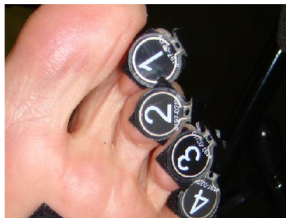
Figure 4 Sensor placement: 1 = Apex of second digit, 2 = Apex of third digit, 3 = Apex of fourth digit and 4 = Apex of fifth digit.
