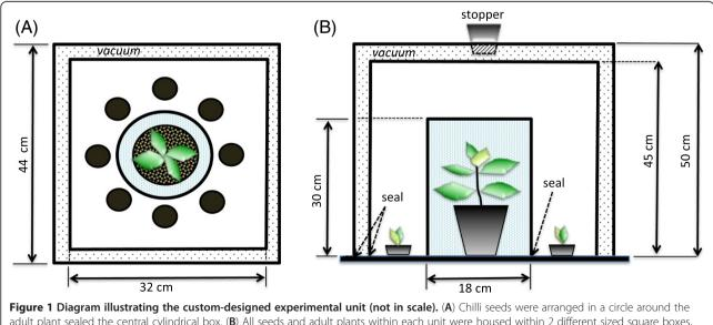
adult plant sealed the central cylindrical box. (B) All seeds and adult plants within each unit were housed within 2 different sized square boxes, one inside the other, with the air in between the two boxes removed using a vacuum pump. This schematic representation has been adapted from [17].
