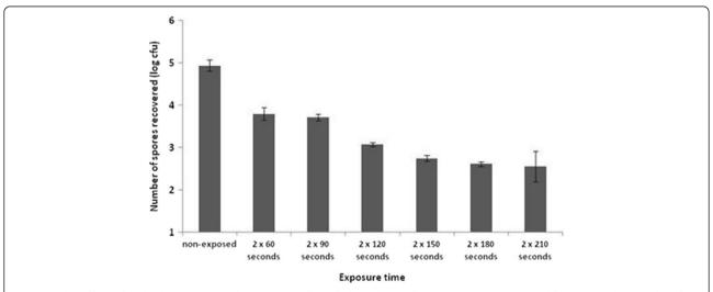
Figure 2 The effect of cycle duration upon the mean number of *Clostridium difficile* 027 spores recovered from a stainless steel surface (n = 5; error bars indicate the standard deviation).
