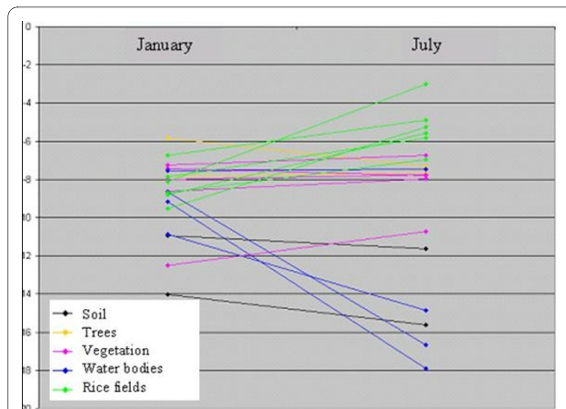
Figure 2 Evolution of backscatter coefficient between ASAR_IMP_1P of January and July 2004. The backscatter coefficient of rice field increased, open water decreased and urban backscatter coefficient remained relatively unchanged.
