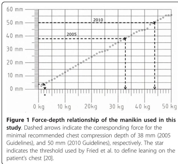
**Figure 1 Force-depth relationship of the manikin used in this study.** Dashed arrows indicate the corresponding force for the minimal recommended chest compression depth of 38 mm (2005 Guidelines), and 50 mm (2010 Guidelines), respectively. The star indicates the threshold used by Fried et al. to define leaning on the patient's chest [20].
