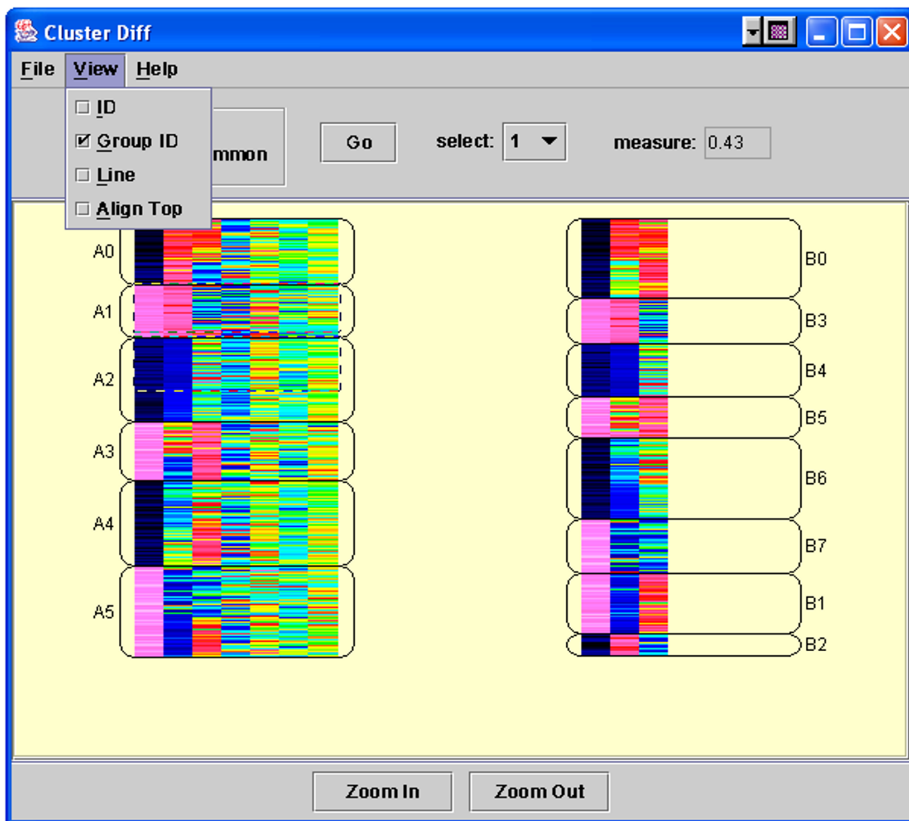
Figure 5 Screenshot of the Cluster Diff window. The main window contains the file, view, and help buttons. In this figure, the left group (A) has 6 clusters, from A0 to A5; the right group (B) has 8 clusters, from B0 to B7. In each cluster, the column represents the dimension of the Microarray data and the row represents the gene's profile. The score is the measurement of similarity.
