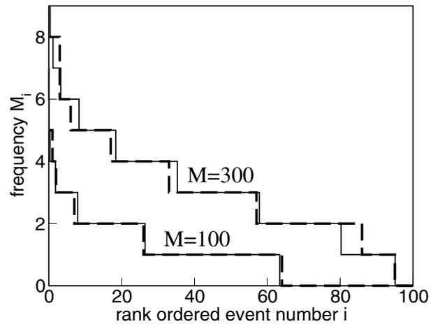
**Figure 3** Rank ordered frequency distribution for  $N = 100$  equally distributed events for different sample size  $M$ . The solid line shows the distribution as predicted by Eq. (5), the dashed line shows the distribution of independently drawn equidistributed random numbers from the interval  $[1, N]$ .
